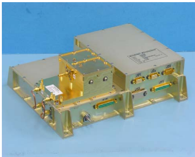
Fig. 2 Engineering model of the RAA GPS POD receiver ([2])
